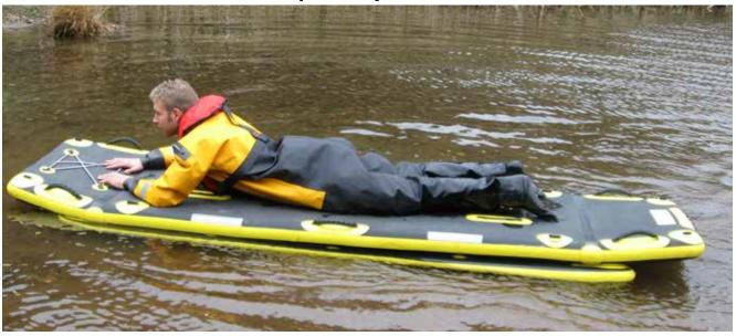
The RP3 is an inflatable platform for the recovery of casualties primarily in shallow water, mud, ice and swamp environments. With catamaran style sponsons, the RP3 provides a stable working platform and with its large, flat, open-toped surface recovering casualties over the side is far simpler than with an equivalently sized rescue sled.
